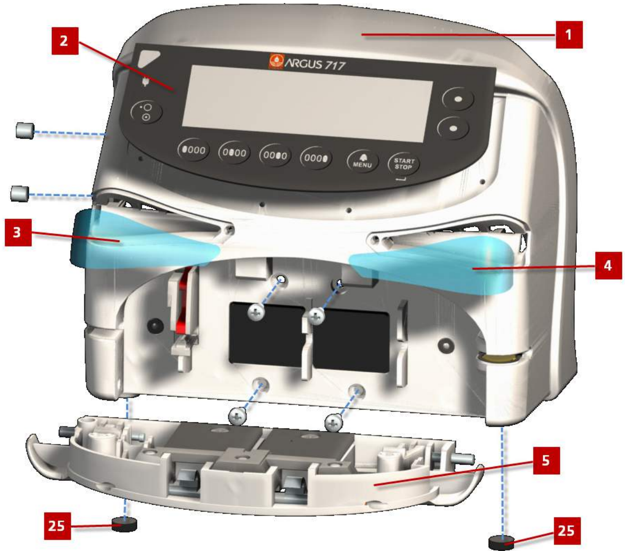
Figure 41: Exploded View ARGUS 71x V - Casing front outside
